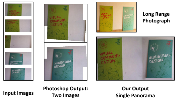
Figure 1: The long range photograph of a scene taken from an SLR camera is shown in top right. When such a scene is probed by a consumer-grade quadcopter, it results in the input images shown on the left (color balance is different from the SLR camera). The state of the art methods (middle column) are unable to make a single mosaic because the vacant space (more than two feet wide as seen in third picture on the left) does not seem to have any matchable features with subsequent input images. Our method handles this situation (bottom right) producing an orthographic view.
